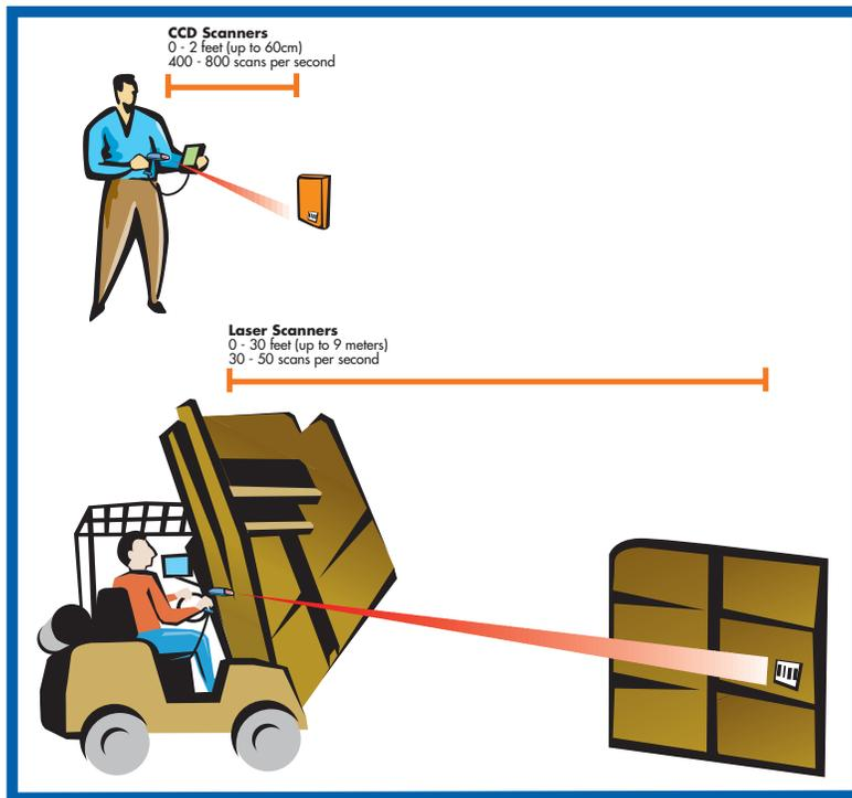
*CCD scanners scan most effectively at shorter distances, but scan at a much higher rate of speed. lasers are ideal for long-range scanning applications.*
